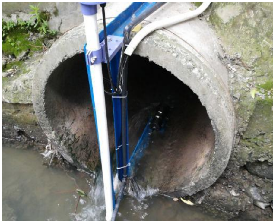
Fig.: 28 Installation Diagram of \Phi 800 mm Pipe
