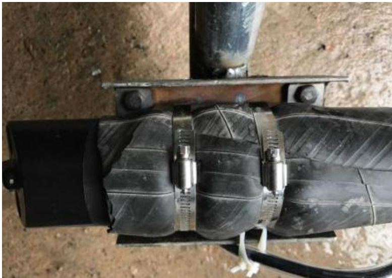
Fig. 34 Fixing the Sensor on Bracket
