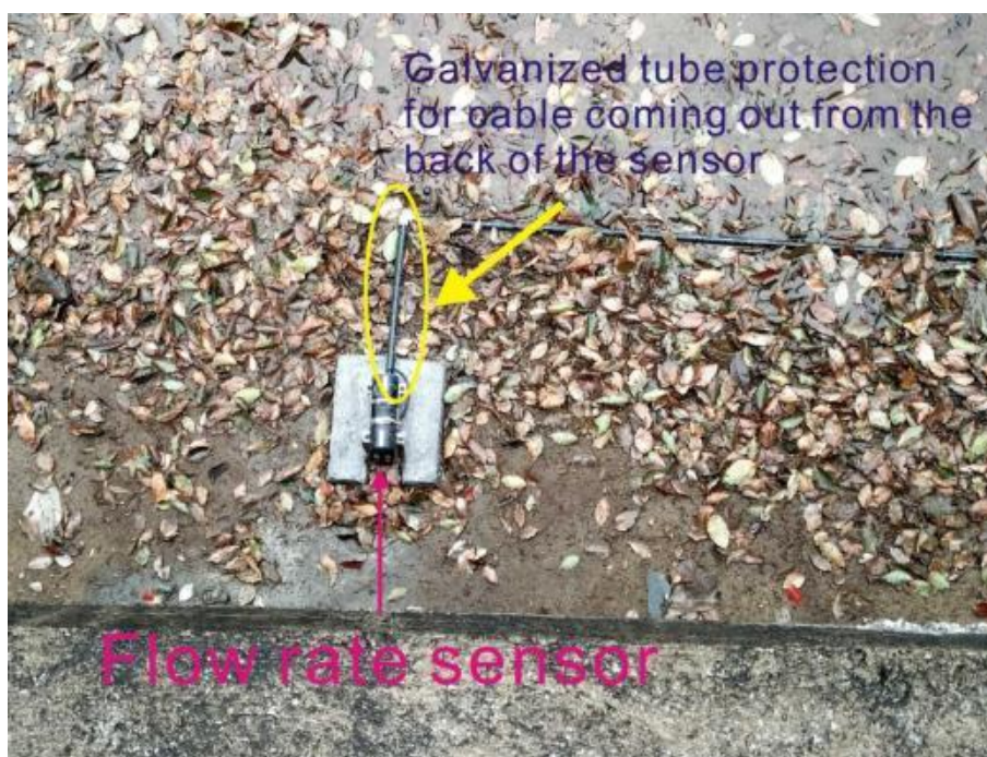
Fig. 20 Installation in Water Cut-off Channel
